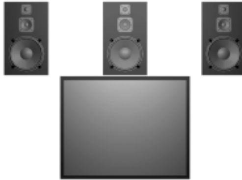
Figure 2-12 Ideal Setup - All Speakers Above Screen
