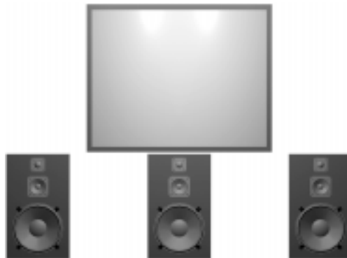
Figure 2-13 Ideal Setup - All Speakers Below Screen
