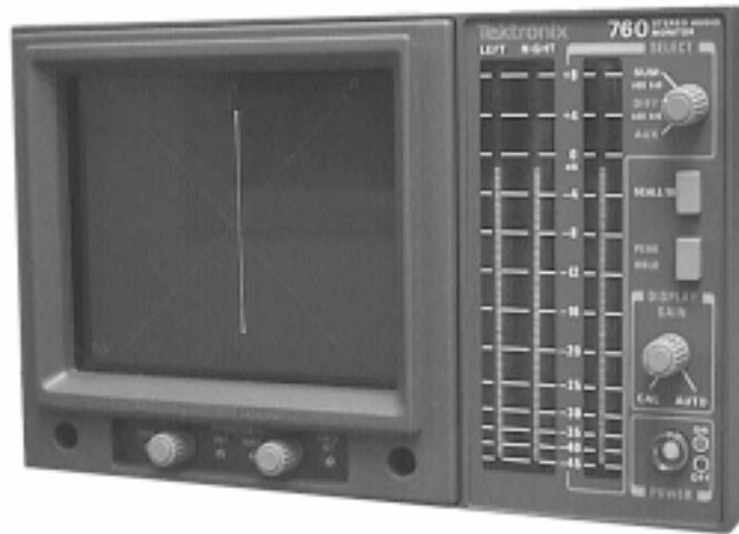
Figure 2-21 Tektronix 760 Phase Scope Display of Center Channel Information
